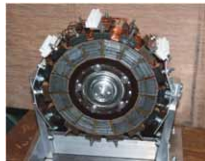
Figure 5 The stator designed and built at Ghent University [6]
