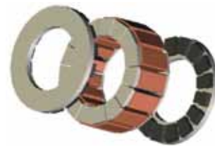
Figure 4 The axial flux PM generator consisting of rotor – stator – rotor [6]
