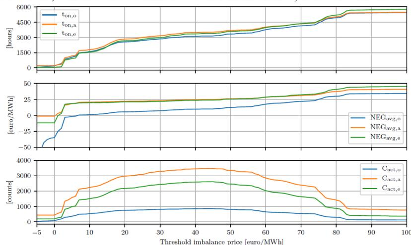
**Figure 7:** The top graph shows the number of hours the electrode boiler would be switched on, the middle graph shows the averaged paid imbalance price and the bottom graph shows the number of times the boiler would be switched on.
