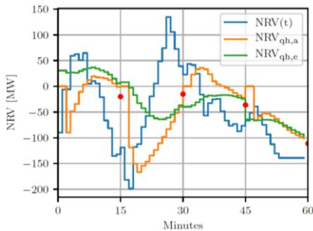
**Figure 4:** In blue the actual NRV values as gathered close-to-real-time, in orange the calculated simple average and in green the calculated heatmap average. The red dots represent the actual validated average NRV for the past quarter-hour.
