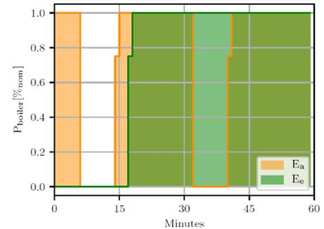
**Figure 6:** Boiler energy consumption with a threshold imbalance price of 20 euro/MWh, in orange for the simple averaged method, in green for the heatmap method.
