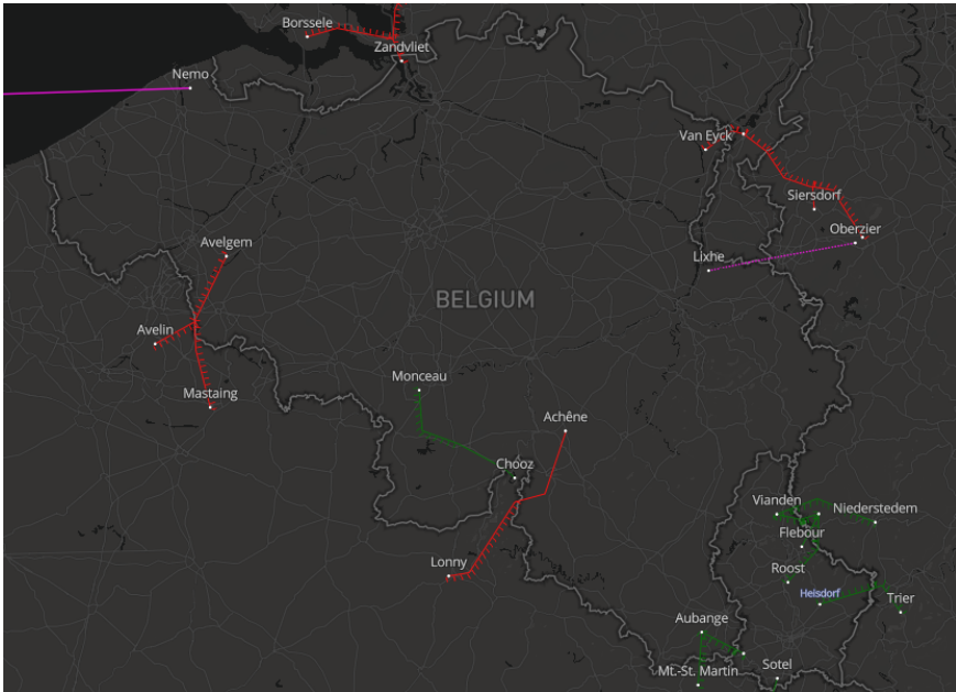
Figure 2.11: Belgian LFC area with the interconnectors. Colours denote technology and voltage levels, with red being 400 kV AC, green being 220 kV AC and pink being DC.
