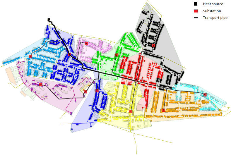
Figure 2.6: Output of a simulation indicating the location of distribution clusters, substations and pipe routes.
